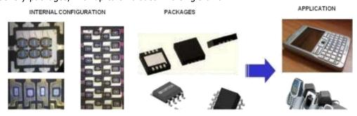
2. Light sensors – These optical devices sense the intensity of light and trigger the automatic switching on and off of headlights and the automatic adjustment of air conditioning settings in cars. The package is a transparent custom-body Quad Flat Pack Leadless Package ("QFN").
