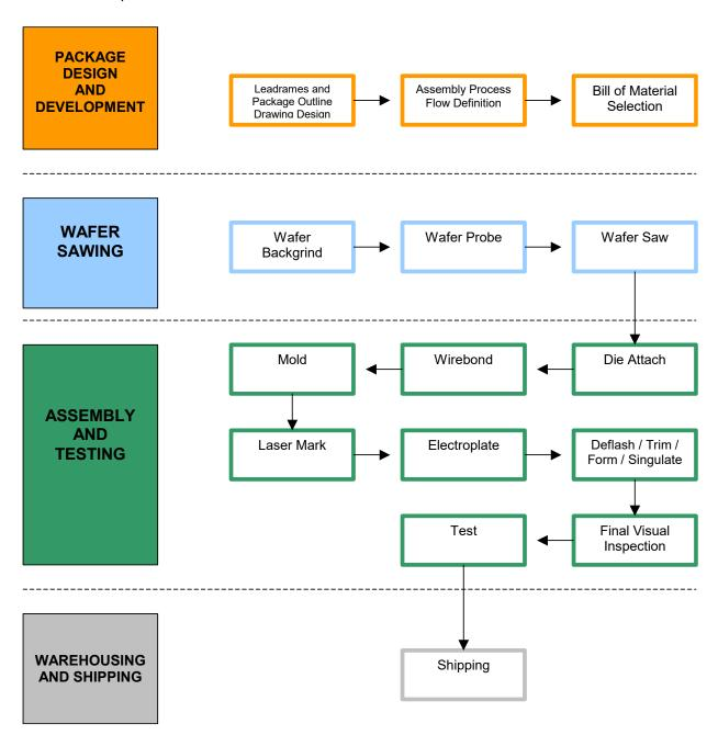
The back-end semiconductor operation starts with package design and development. The design phase pertains to a.) the determination of the type of package to be used that conforms to industry standards,
