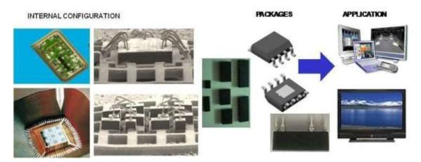
6. Power management devices – These devices are used in a wide range of power management applications from telecommunications, industrial equipment, portable devices, computers, and networks. These are packaged in SOIC with the die pad exposed.
