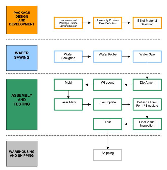
The back-end semiconductor operation starts with package design and development. The design phase pertains to a.) the determination of the type of package to be used that conforms to industry standards, b.) the substrates that will match the intended package, and c.) the material set that will be used to meet customer specifications. This is followed by tooling selection and ordering.
