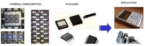
2. Light sensors – These optical devices sense the intensity of light and trigger the automatic switching on and off of headlights and the automatic adjustment of air conditioning settings in cars. The package is a transparent custom-body Quad Flat Pack Leadless Package ("QFN").
