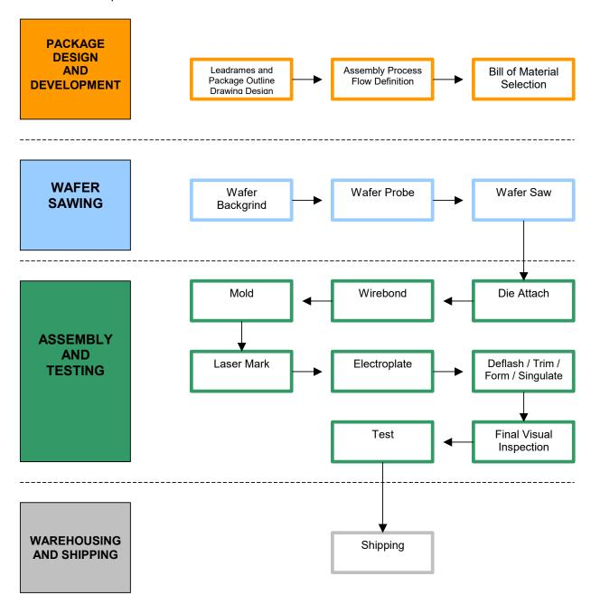
The back-end semiconductor operation starts with package design and development. The design phase pertains to a.) the determination of the type of package to be used that conforms to industry standards, b.) the substrates that will match the intended package, and c.) the material set that will be used to meet customer specifications. This is followed by tooling selection and ordering.
