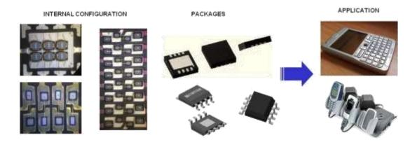
1. Light sensors - These optical devices sense the intensity of light and trigger the automatic switching on and off of headlights and the automatic adjustment
